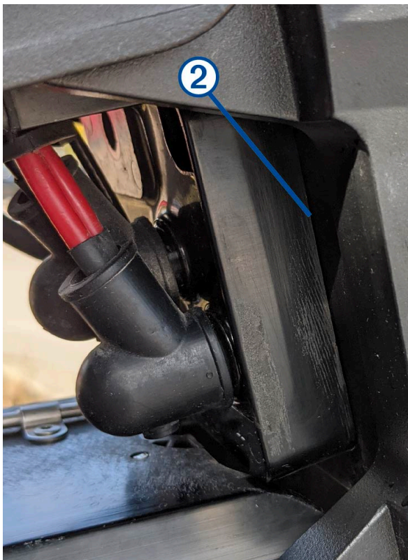
Motor without the Seal Installed
